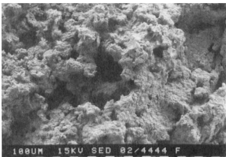
FIGURE 7 SEM : DWM Tablet Interior After Six Hours Intrinsic Dissolution At 50 rpm
